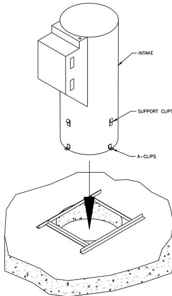
4. After first intake section has been set, slip the beaded end of the plain chute section ("b" section) into the intake section making sure it is sealed all around. Some floor heights may require multiple "b" sections. Check with level to plumb chute as installation proceeds.
