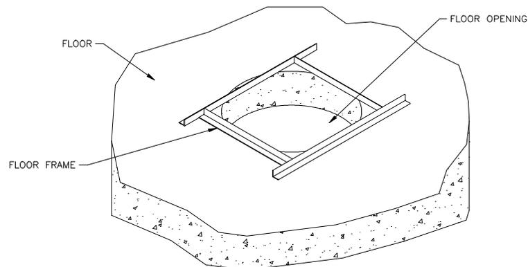
3. Set the first intake section, this section has 4 a-clips with slots welded to the bottom of it, into the floor opening and seat the support clips over the floor support.
