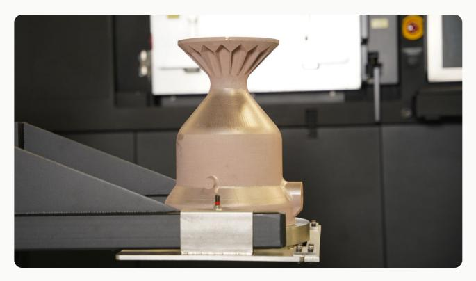
Regeneratively-cooled rocket thruster printed in GRCop-42. The thruster is a development unit that will demonstrate the first ever flight of large liquid modular aerospike rocket engine and gather crucial operational and performance data in a relevant sub-orbital trajectory. The part--which went through DfAM but was unable to print on a conventional metal AM system-- was printed on its first attempt using a Velo3D Sapphire.
