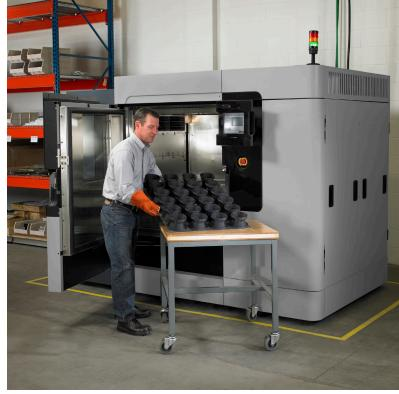
FDM technology is manufacturing-ready, with the most build volume for large parts or multiple smaller parts.
