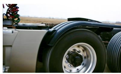
Minimizer put their ULTEM 9085 resin material prototype fenders through real-world functional testing.
