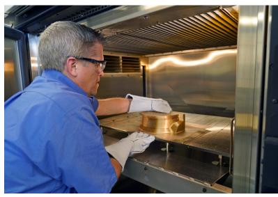
Team Penske counts on the reliability of FDM technology to help them win races, producing race-ready car parts and tools like this composite lay-up mold.
